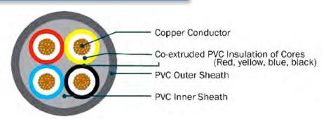
ALOKE Submersible Cables are suitable for submersible pumps motors. Our doublesheathed round cables are better suited for heavyapplications like duty sewage, slurry and dewatering pumps. The
