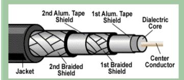
ALOKE COAXIAL cables are used as a distribution cable for indoor CATV, CCTV systems and as a connection cable for satellite systems where lower attenuation required. ALOKE Cable can provide for all your video, audio and data needs. For long-length, backbone applications, Coaxial Cable is ideal for entry point feeder systems running to a building and extending to each floor and room of a commercial or residential building.
