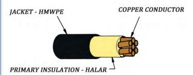
ALOKE Cathodic protection cable is especially suited for deep anode lead wires. OUR CABLE is inert to reactive compounds and has an outstanding ability to prevent the passage of gases and also extend the life of deep anode installations. The cable is composed of stranded copper wire covered by two layers of insulation
